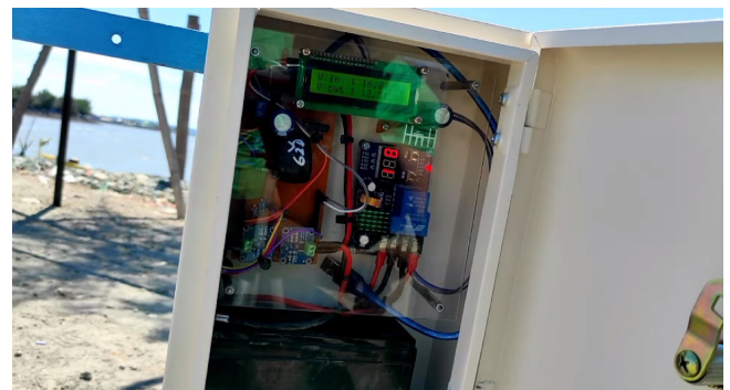
FIGURE 15 Charge controller integration test
