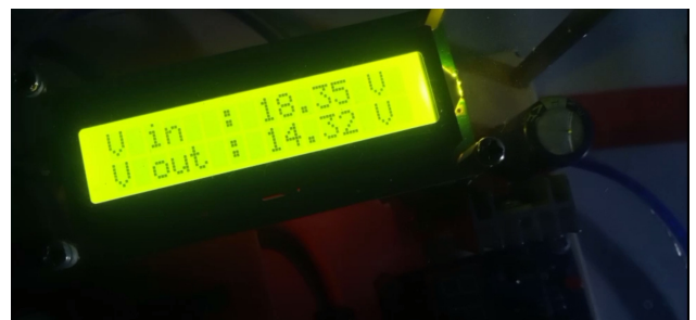
FIGURE 5 Open-loop buck converter test
