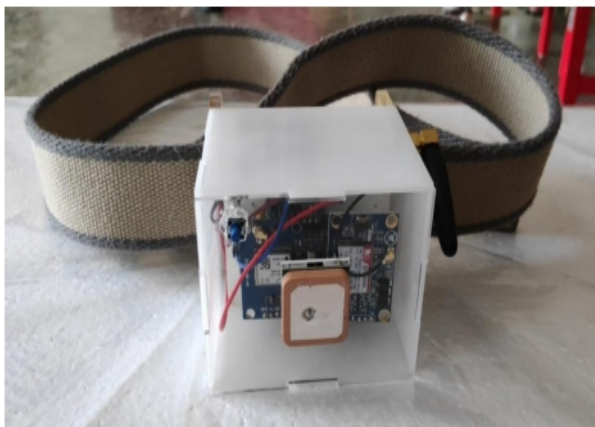
FIGURE 4. Tool Prototype Design of The portable tools of the elderly Alzheimer's patient
