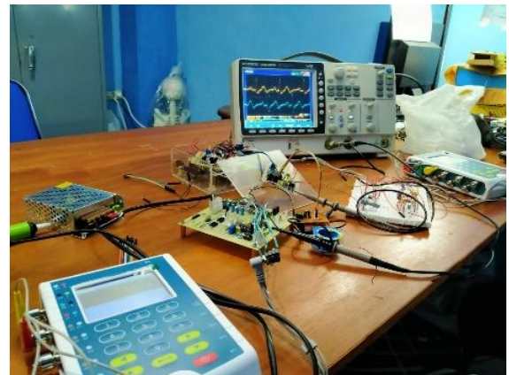
FIGURE 7. Experimental ECG signal displayed on an oscilloscope using two phantoms to test two instrumentation amplifiers.
