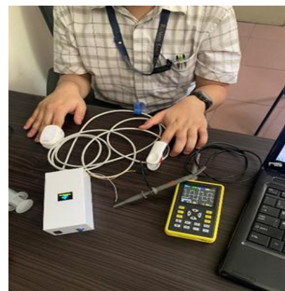
FIGURE 4. Demonstrating methods of data collection, and concurrent measurement using designed modules and standard tools. The index finger of the right hand was measured with the module and the index finger of the left hand was measured with a standard instrument.
