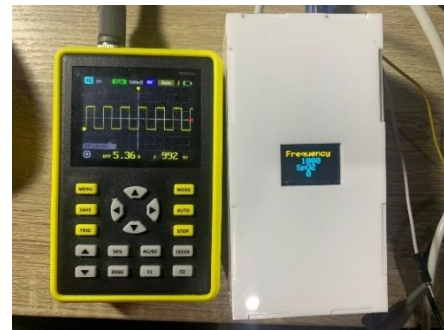
FIGURE 3. The results of the design of the SpO2 tool with an OLED LCD, on the right. Meanwhile, the left is a digital oscilloscope which is used to determine the capability of the flip-flop frequency generator
