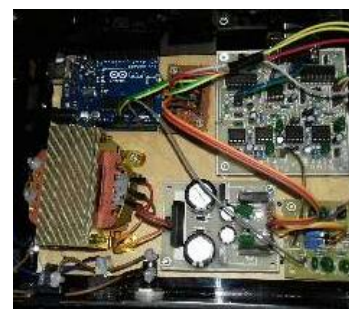
FIGURE 5. Module Design consists of an analog signal processing circuit, power supply, and a microcontroller circuit.
